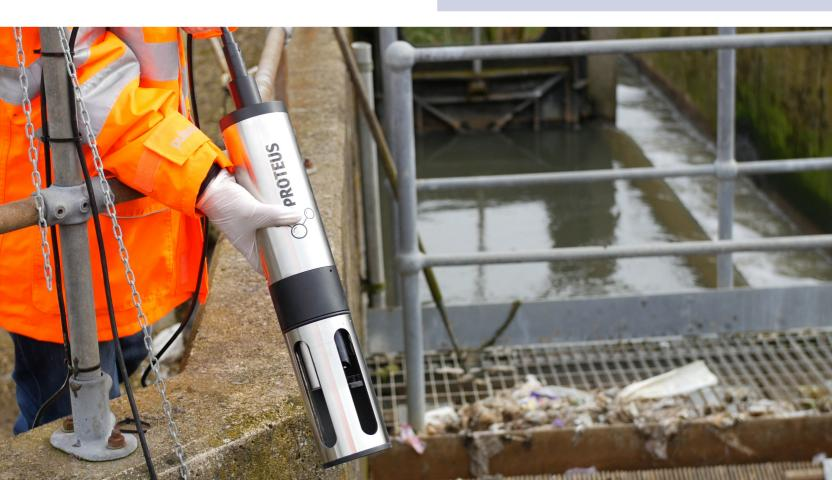
**Self cleaning:** As it is essential that optical sensors have a cleaning mechanism, the Proteus is also supplied with an integral wiper which cleans all of the Proteus' sensors before every measurement cycle.
