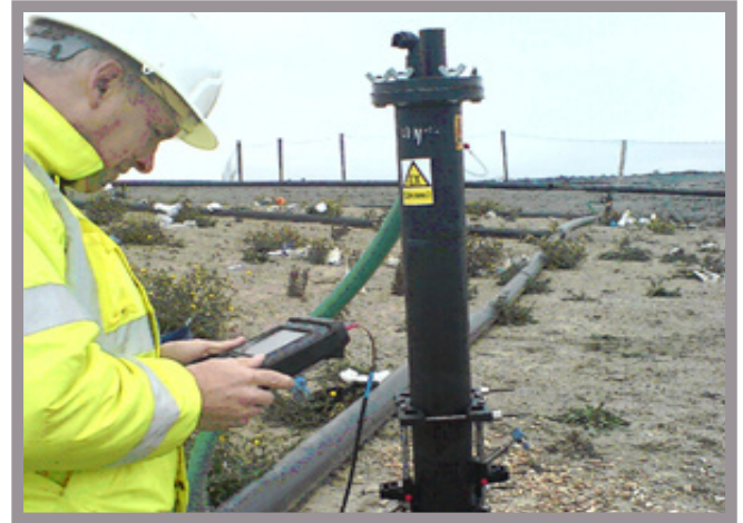
fig2. PT878GC used to measure landfill gas
